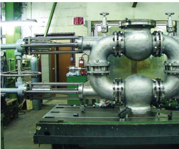
Fig. 8 – Offshore tandem changeover valve with rupture discs
